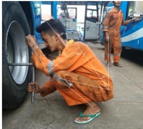
**Figure 6.** Wheel nut installation *Source : Documentation result, 2018*
