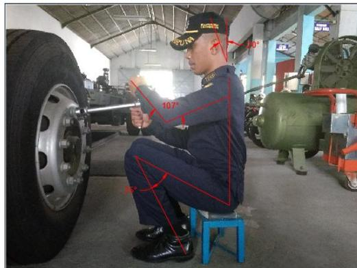
**Figure 9.** Wheel nut installation by using chair.
