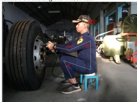
**Figure 10.** Locking the wheel nut by using chair.
